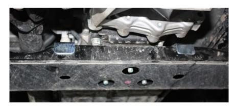
3. Slide (UGNPR51T2) under the front guard (UGNND40F1)
