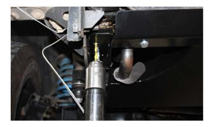
4. Using a 19 mm drill bit drill a hole in the chassis (as shown below), drill out the pre existing hole on the passenger side chasses rail (as shown below)
