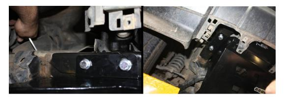
6) The rear of the guard can also be bolted up to crossmember. M10 bolts have been supplied to bolt up to captives on crossmemeber. Shown Below.
