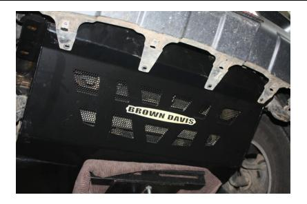
8) Factory Plastic Bumper shield can now be bolted back up into place. Shown below.
