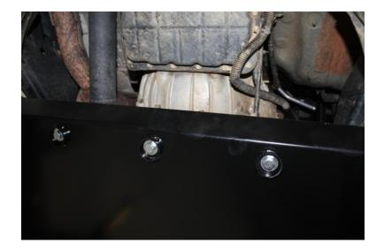
7) Factory bumper can now be bolted to captive threads in front of guard.
