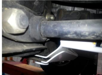
3. Fit 2x **SET SCREW – HEX – M10 X 60mm – PLATED 8.8**, with spring and panel washers, into the holes in the center of the guard.
