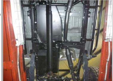
33. Double check all fuel line clamps and make sure fuel lines are secure and not rubbing on tank or body of the vehicle. Road test and check for rattles & squeaks.
