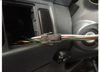
31. Connect the white plugs from both the BUZZER – PEEL – CP 5 and the WIRE – TWIN CORE – 3.0mm – BROWN/WHITE—WITH PLUG.
