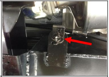
25. Use the P shaped brackets on the wings of the tanks to support the hand brake cable.
