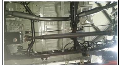
2. Cut the plastic knobs off the fuel line clips.
