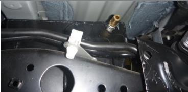
20. Using the HOSE – FILLER – 35mm join the two tank tubes.
