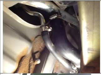
Step 16. Re-fit exhaust being sure to check clearance to tank bracket. Some aftermarket exhaust may need to be slightly relocated.
