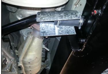
14. Double check all fuel line clamps and security of fuel lines. Fill tank and double check all fuel system for leaks. Road test and check for rattlers & squeaks.
