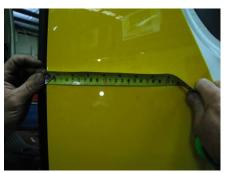
On the inside of the vehicle measure and mark 480mm vertically from the bottom sill and slightly right of centre. Ensure the measurement that is marked is not outside the indentation on the panel as indicated in the photo below.
