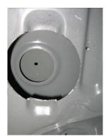
The outside hole needs to be cut. Using a 57mm diameter hole saw cut a hole around the hole centre. Use a dye grinder to notch the hole at the top, as indicated by the photos below, so the fuel filler can be inserted easily.
