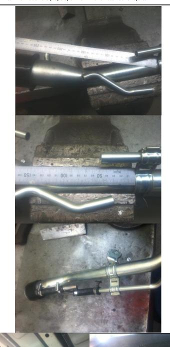
4. Reinstall modified filler tube to the original location.
