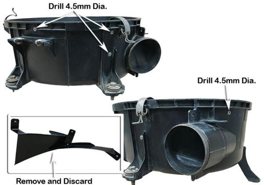
Using the body saw cut-off the 3 tabs which retained the pre-spinner section to the air cleaner base inlet.
