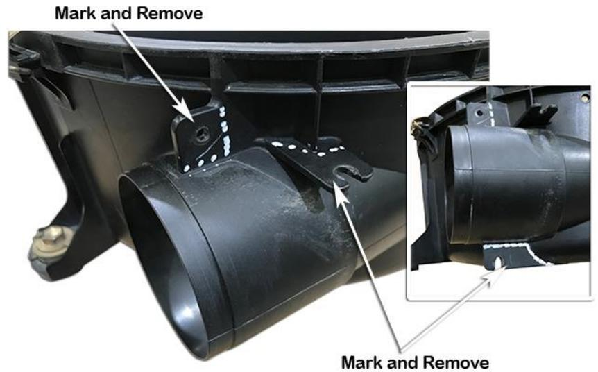
Using a paint pen, mark a cut line around the base of the inlet snout.
