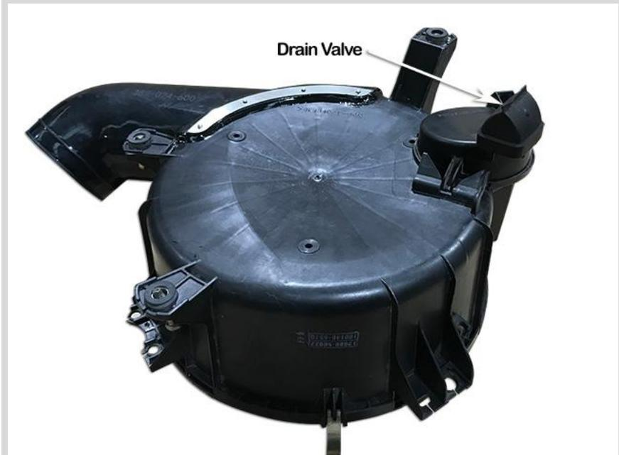
The installer should also check the condition of both the Air Cleaner Lid Seal and the Dust Cap Seal, if necessary, these items should be replaced if they are in a poor serviceable condition.
