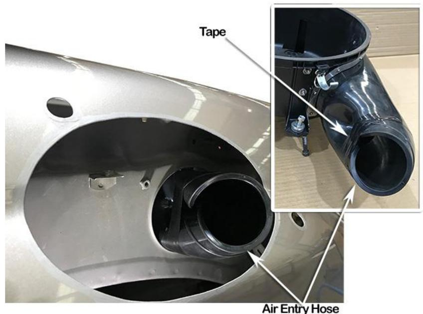
Loosely install the 100/120mm hose clamp (item 17) loosely over the air entry hose (Item 10).
