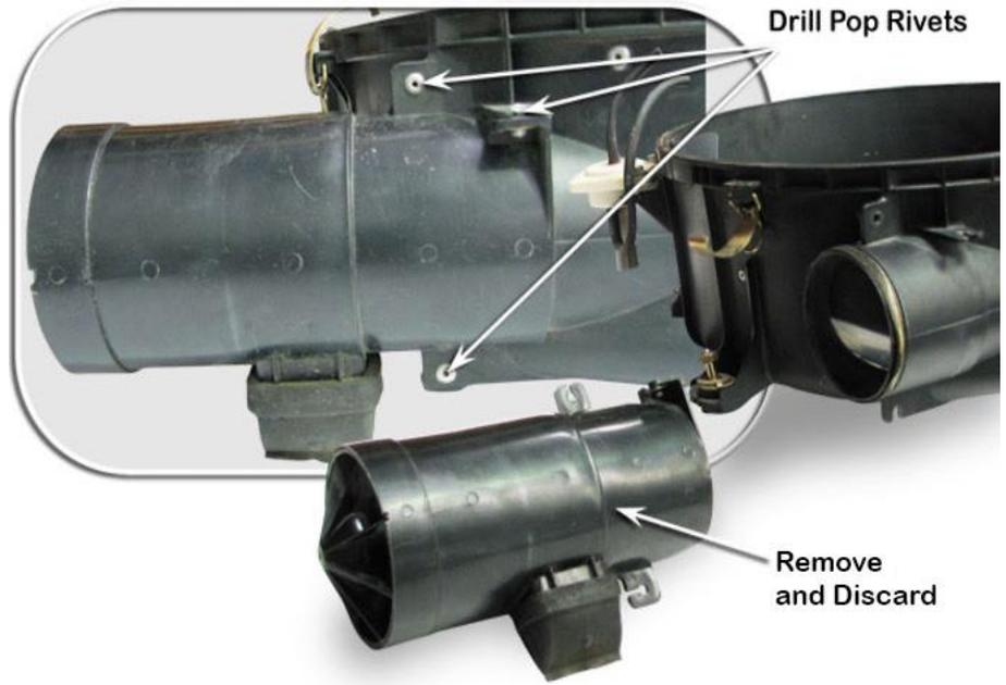
Using a 4.5mm drill bit, drill out the four pop rivets retaining air deflector in the air cleaner base (hold the back of the pop rivets with a pair of pliers to prevent them from spinning whilst drilling out the pop rivets).
