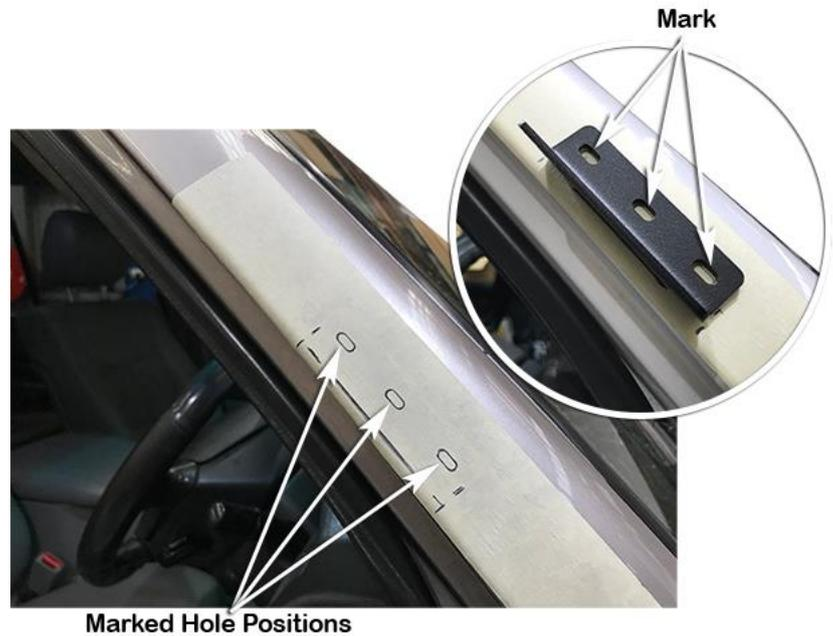
Drill a pilot hole for each of the three marked hole positions in the centre of each marked slot.
