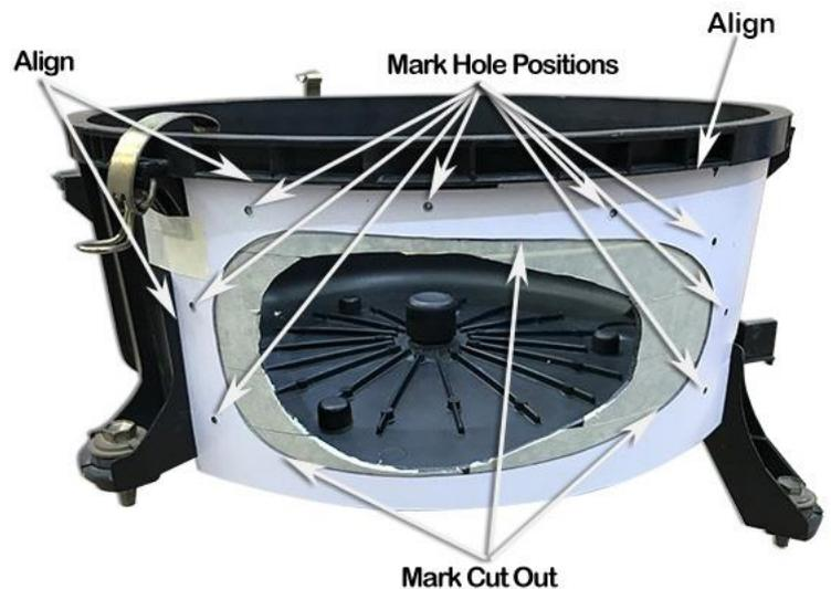
Using a 4.5mm drill bit, drill all eight marked hole positions.
