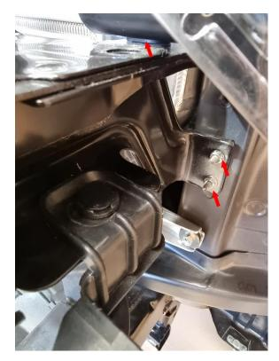
15. Remove both horn brackets and place over the top of the radiator out of the way. Unbolt 2 x upper and 2 x lower bolts from bonnet latch upright, removing as a complete assembly. Unclip all 3 harness clips and bonnet release cable and place out of the way for easier OEM intercooler removal and to avoid damage to air conditioning condenser directly behind.
