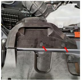
5. Remove 11 x scrivets indicated with red arrows to allow access to 2 x phillips head screws which need to be removed, indicated by green arrows. The rubber weatherstrip near the headlights may need to be lifted to allow easier access to removing the scrivets.
