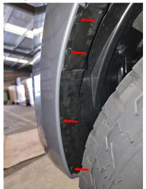
10. Move the passenger side wheel arch liner away from the bar enough to gain access to inside the front bar to release both wiring harness connectors with a narrow flat blade screwdriver.
