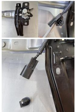
24. The harness bracket on the passenger side of the bonnet latch support needs to be bent to allow clearance. A small cut (indicated by yellow line) will allow this to bend flat as shown.
