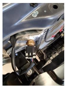
17. Loosen all 4 hose clamps on hot and cold side intercooler hoses. Remove top 2 x nuts and lower 2 x bolts on intercooler. The intercooler can now be removed. Remove hoses if hard pipe kit has also been purchased. Press out steel inserts before removing rubber bushes from OEM Intercooler to be reused.
