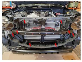
Remove front bumper bar support by removing 6 x nuts and 2 x bolts securing the headlights. Unclip sensor before removing.
