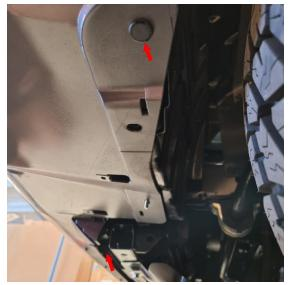
Remove 4 x small scrivets inside each wheel arch area carefully, as these are prone to breaking easily.
