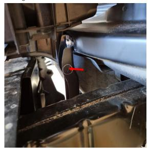
Remove 8 x scrivets securing both upper driver side & passenger plastic ducts and entire lower plastic duct. The ducts can all be removed.
