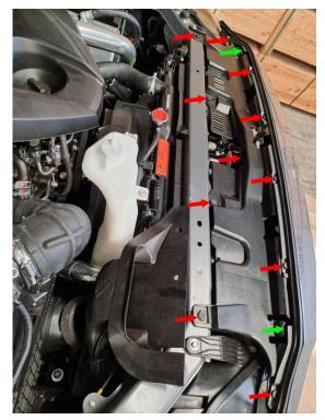
Remove 4 x scrivets from inside the grille and 1 x phillips head screw from inside the badge.
