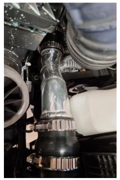
29. With Plastic engine cover removed, loosely fit the cold pipe onto the intake manifold of the engine with the other end close to the opening on the passenger side of the radiator
