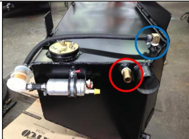
5. Using thread sealant install the 2 BRASS FITTING-TAIL BARB – 5/16" x 1/8" BSP to the FUEL PUMP – POSI-FLO.
