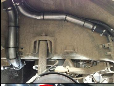
25. Connect the **HOSE – FUEL AND EMISSION - 8mm** that is connected to the pump to the smallest pipe on the **TWIN FILLER.**
