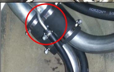
26. Using the remaining HOSE – FILLER – 48mm and hose clamps connect the FILLER TUBE between the TWIN FILLER and the auxiliary tank
