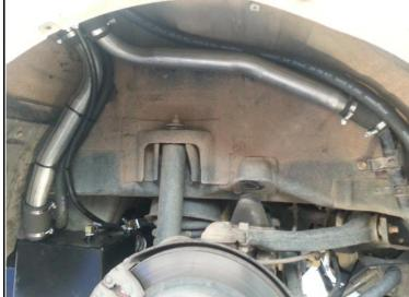
27. Connect the **HOSE – FUEL AND EMISSION - 8mm** that is connected to the pump to the smallest pipe on the **TWIN FILLER.**
