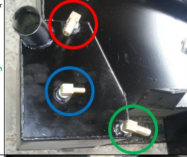
4. Install the **BRASS FITTING-TAIL BARB— 1/2" x 1/4"** BSP in remaining socket, **Circled in red.**
