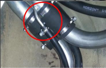
28. Using the remaining HOSE – FILLER – 48mm and hose clamps connect the FILLER TUBE between the TWIN FILLER and the auxiliary tank
