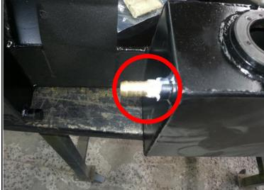
5. Using thread sealant install the 2 BRASS FITTING-ELBOW- 1/8" x 5/16" BSP to the FUEL PUMP - POSI-FLO so the barbed tube runs parallel with the base plate
