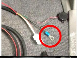
9. Connect the plugs from the **FUEL GUAGE/SWITCH – CP 309GS LED DASH UNIT** to the **LOOM WITH BUZZER.**
