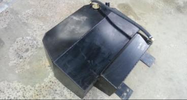
16. Fit the supplied mounting bracket to the existing holes at the front of the spare wheel cavity using M10 hardware supplied.
