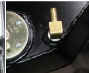
15. Fit the HOSE - FUEL AND EMMISION - 16mm to the BRASS - ELBOW - 5/8" x 3/8" BSP fitted in previous step.
