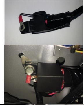
Connect the plugs from the FUEL GUAGE/SWITCH – CP 309GS LED DASH UNIT to the RELAY/BUZZER – PEEL – CP 5.
