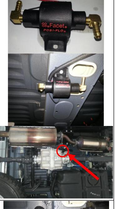
Using HOSE – FUEL AND EMISSION - 8mm install the FUEL FILTER – INLINE – 8mm to the suction side of the pump.
