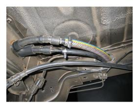
5. With the sender unit fully connected, align the mounting brackets with the factory holes and raise the tank to meet the mounting position. Using the factory bolts removed from the standard tank, re-install all bolts.
