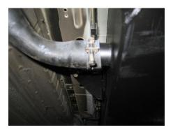
9. In order to check for potential leaks in the installation, only fill the tank up to a maximum of half a tank and test drive the vehicle for a short period, before re-inspecting the entire installation looking for any leaks at the hose connections on both the tank and filler. Again, check mounting bolts are firmly fastened prior to completion.
