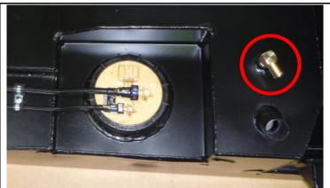
10. Fit filler and fast fill hoses to the new tank. Take note of the position of the hoses before removing them from the standard tank. Fit hoses to the new tank in the same orientation as they were removed from the standard tank.
