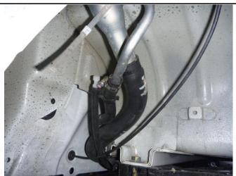
2. Lift car on hoist or jack stands to remove the fuel tank. Unclip fuel lines at front of tank making sure lines don't syphon fuel onto the ground.
