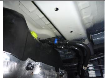
3. Undo front and rear mounting straps from under the tank, keeping bolts to be used on the new tank. Lower tank down carefully, only far enough to gain access to fuel pump/sender unit wiring, unclip plug from gauge, then lower the tank to the ground.
