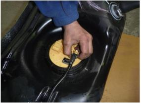
5. Remove fuel sender unit. This requires a special tool. In the absence of the special tool, the sender outer ring can be undone using a hammer and a blunt piece of metal or wood used as a drift. Tap lightly on alternating sides of the ring changing ribs regularly to avoid breaking ribs
