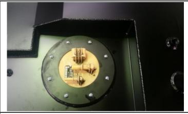
7. Fit the fuel lines to the new tank. Fit the cushion clamps to hold lines in place and then tighten using M6 nuts and washers supplied.
