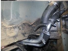
4. Fit 5/8" x 5/8" x 5/16" TEE PIECE to the lower part of the fast fill rubber hose, close to the tank.
