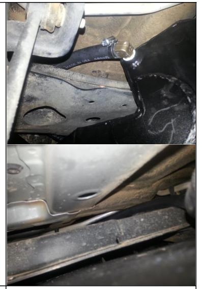
22. Double check all fuel line clamps and security of fuel lines. Fill tank and check for leaks. Road test and check for rattles & squeaks. Re-check for fuel leaks.
