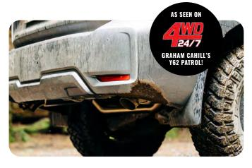
Both of Torqit's twin exit options for the Y62 Patrol fit with a 35" spare tyre; the key difference is the exhaust note. Our loud option produces an aggressive V8 note, while our touring option provides a more subtle sound that is ideal for long distance driving and towing.
