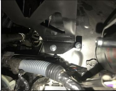
Earlier removed bolt (1) can now be used to secure lower end of bracket-brace
