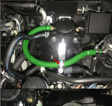
Reinstall hose clamps and ensure all are secure
