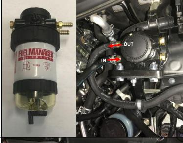
Use the supplied fuel hose (1) to connect the fuel filter as pictured
