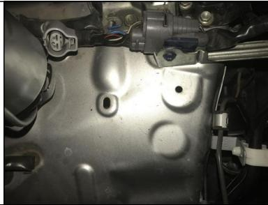
Fasten filter bracket-base to chassis holes
