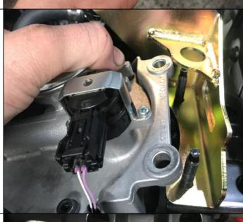
Use the socket hole to secure the sandwiched assembly back in place with the factory nuts.
