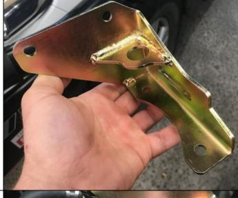
Unscrew the nuts securing the factory fuel filter in place. Lift as shown, and thread the Brown Davis (BD) bracket over the captive bolts, then return the factory fuel filter over the top.
