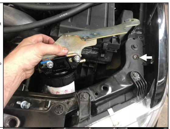
Fit the FF-NND40 into the engine bay (pass side) as shown here. Loosely place the removed factory nut.
