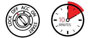
NOTE: For vehicles with push button start feature, ensure the key fob is moved >10m away from the vehicle so as not to activate accessory power.
