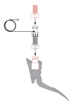
Connect the EVC unit in-line between the factory plug and pedal assembly. Ensure the plugs are aligned correctly to prevent damage to the internal pins. Do not use excessive force to push the connectors together. Any resistance may indicate there is a pin missalignment which may cause damage to the unit.
