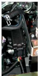
If relay for bull bar lights fitted, re-fit to computer bracket as above
