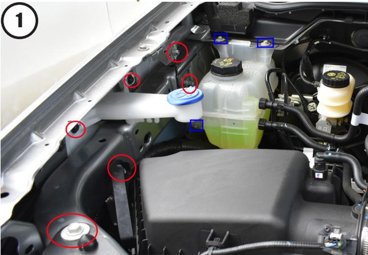
**3).** Check earth wire is sitting in the groove of the perimeter beam, refit original bolt and tighten. Tighten three coolant expansion mounting bolts if they were loosened previously.
